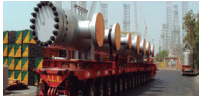
56 inches cladded manifold
